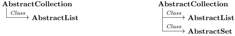
Figure 2: Two trees that can be distinguished by counting the number of children the root has.
